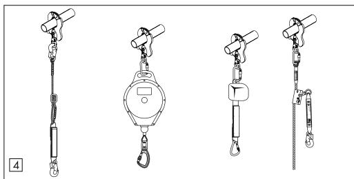
Connect the energy absorbing / connecting element to the snap hook (e.g. energy absorber with lanyard, retractable fall arrester, working lanyard, or rope grab).
