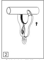
Push the hand grip until the full spread of the clamp, then secure the clamp on the element.
