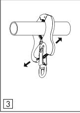
Release the hand grip, enabling the device to automatically secure on the bar.
