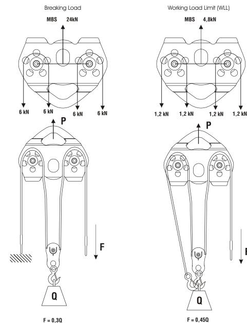
One or more sheaves mounted in a block or a body, which can be used to link a rope (in accordance with EN892 and EN1891) or an accessory cord (in accordance with En564) to a connector (in accordance with EN 12275) to safeguard a mountaineer, and which reduces the friction while the rope or accessory cord is moving under load.
