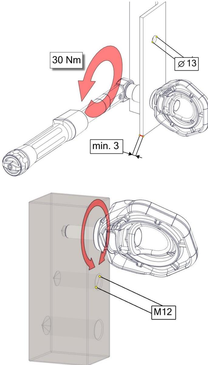
**Figure 4. Installation of anchor point**
