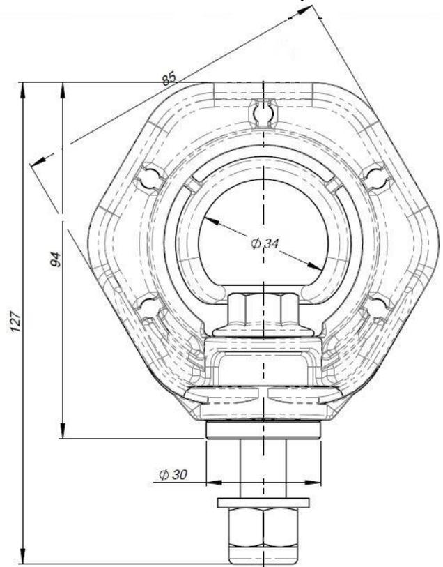
**Figure 2. Overall dimensions AT185**
