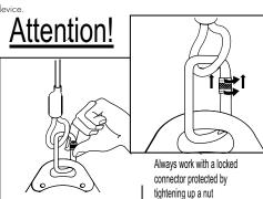
Using the anchor device AT192 in connection with fall arrest system must be compatibile with use instructions of the fall arrest systems and obligatory standards: -EN 361 - for safety harness; -EN 353-2, EN 355, EN 360 - for fall arrest equipment. -EN 362 - for the connectors.
