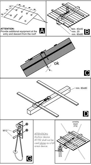
Using the anchor device AT 192 in connection with fall arrest system must be compatibile with use instructions of the fall arrest systems and obligatory standards:
