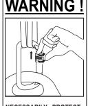
NECESSARILY PROTECT THE SNAP HOOK GATE WITH THE LOCKING GEAR
