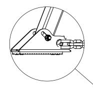
MAXIMUM LOAD TRANSMITTED FROM TM 9-W TO THE STRUCTURE / LOADING DIRECTION Surface, where the TM 9-W safety tripod was placed on must support the max. device load of 12 kN. Loading direction: perpendicular to the surface on which the TM 9-W safety tripod is placed.
