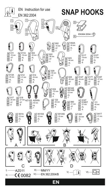
Snap hook is a component of the personal protective equipment against falls from a height. Snap hook must conform to EN 362 - Personal protective equipment against falls from a height - connectors. Snap hook is the openable device used to connect components of fall arrest equipment into complete fall arrest system.
